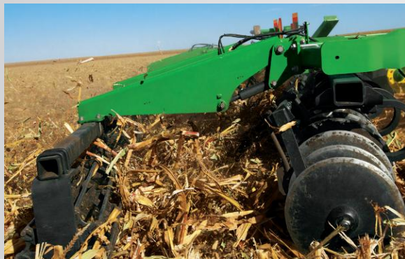
Hefty front blades effectively chop and size residue, manage weeds, and remove field ruts. Meanwhile, the wavy rear blades work to mix and aerate the soil while anchoring residue.
